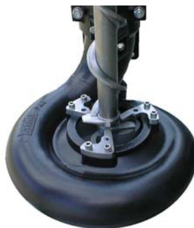
Chopping knives of hardened steel and auger conveyor assure that solids are shredded and thus eliminate pump inlet clogging.
